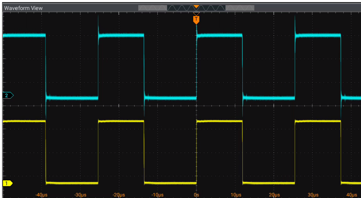
Figure 4. Full low-side gate waveform at 20 V bus voltage. The differential probe exhibits increased baseline noise compared to the optically isolated probe.
