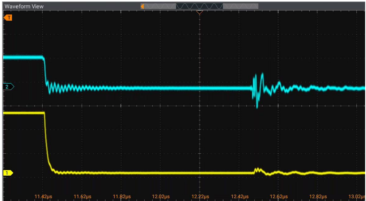
Figure 10. High-side gate falling transition at 20 V.
