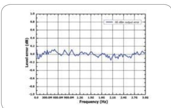
Measured at -110 dBm,level error vs.frequency
