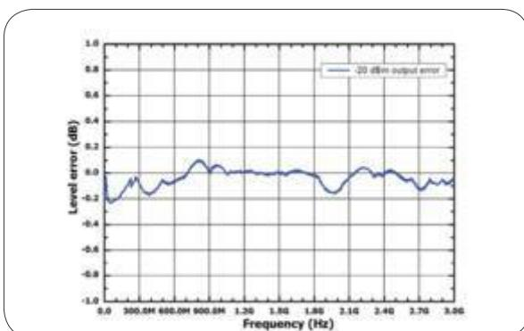
Measured at -60 dBm,level error vs.frequency
