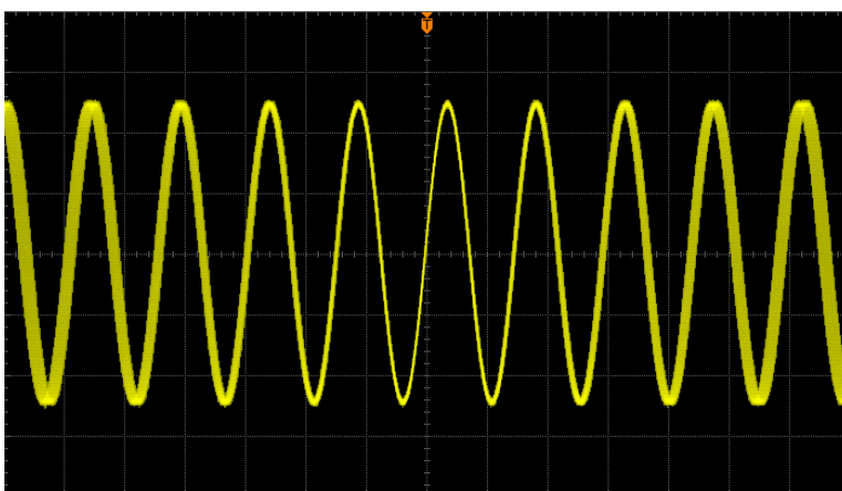
Figure 11-1 Set the Persistence Time of the Oscilloscope to Min
