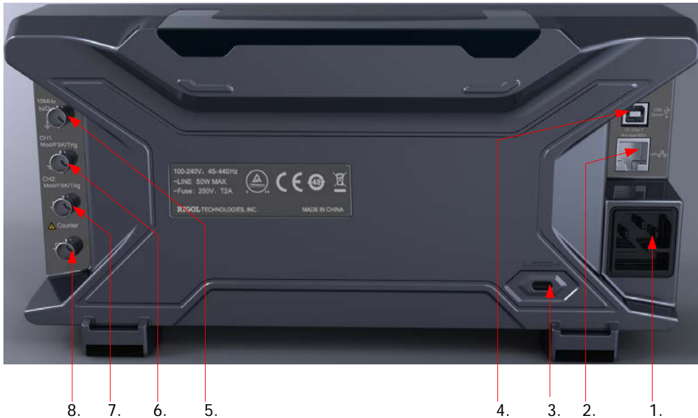
Figure 1-6 DG4000 Rear Panel
