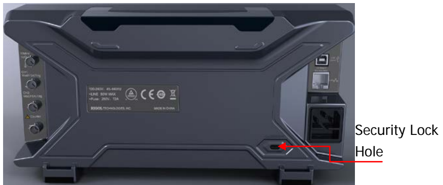
Figure 1-9 Security Lock Hole
