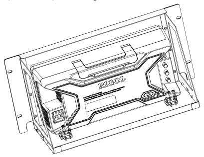
**4.** Load into the machine cabinet: mount the rack with instrument fixed into a standard 19-inch machine cabinet using four M6 screws and square nuts.
