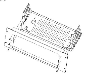
**3.** Place and fix the instrument: place the instrument into the confined position on the support board. Aiming the instrument front panel at the opening of the front panel of the rackmount kit and fix the instrument with four spring washers, four washers, two retaining brackets and four M4 screws.
