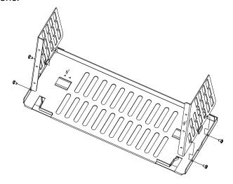
**2.** Install the front panel: let the screw holes fit well together and fix them with six M4 screws.
